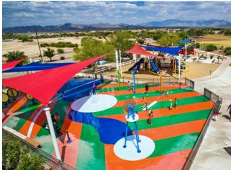
Above: The windmill toy, with its spinning blades releasing constant streams of water, was originally going to be located under the canopy. Though the shade structure was designed tall enough to accommodate its height, water from the windmill splashed and collected on top of the canopy. In a seamless move, the water tower took its place.
